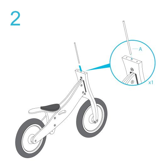
The Mocka Balance Bike has been pre-assembled already. The seat is in the lowest position for a beginner rider. To complete the assembly position the frame and fork of the bike together.
